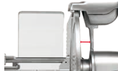
Increased gap between blade and machine body
