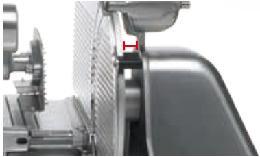
Increased gap between blade and machine body
