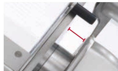
Increased gap between blade and machine body
