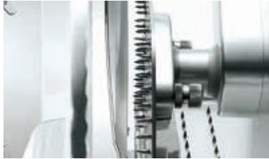
Reduced gap between blade and end weight
