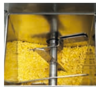
Mixing hopper designed to better knead pasta dough
