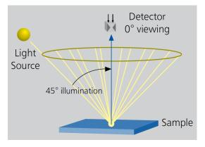
When using an instrument that utilizes a sphere, you will have the option to capture all reflections—both the specular and diffuse reflectances. You also have an option to exclude the specular reflectance. When choosing this latter option, the spherical instrument will generate values very similar to a 45/0 instrument.
