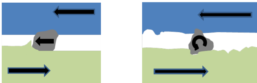
Figure 3 – 3-body abrasive wear mechanisms
