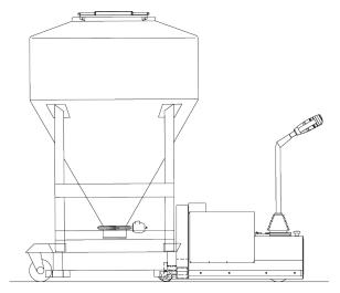
Version with *lifting* from the bottom: This is used when your vessel/bin has 2 fixed wheels
