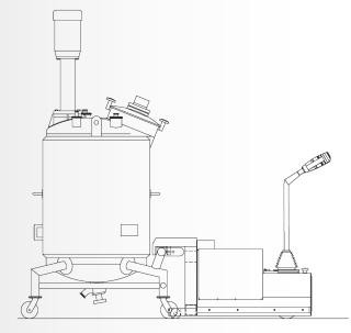
Version with *lowering* from the top: This is used when your vessel/bin has 4 swivel wheels
