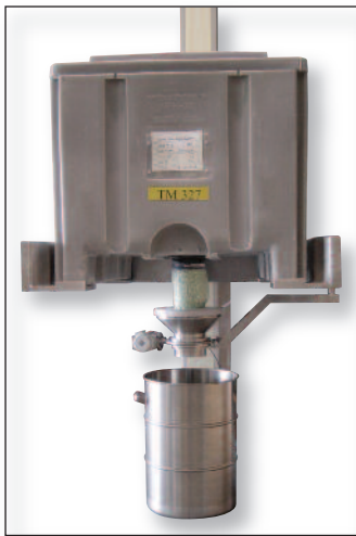
Loss-in-weight tablet IBC discharge to drum
