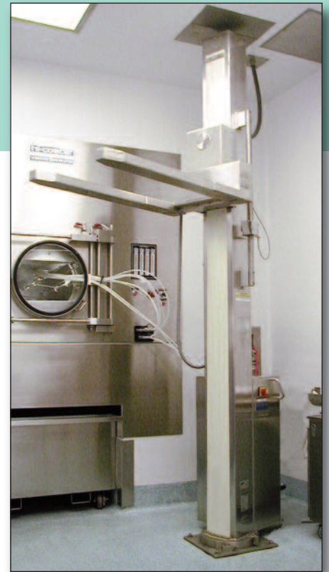
FIBC (supersack) tablet unloader with transverse moving over Thomas Containment Coater inlet.
