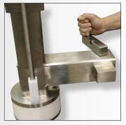
Optional swivel unit: pull out bar, insert into hole and rotate unit. Replace bar and unit is locked into position.
