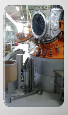
DRUM IRIS FLEXIBLE REACTOR CHARGING INSTALLED ONTO AN OPEN MANWAY SUPPORTED BY THE DRUM IRIS LIFTER.
