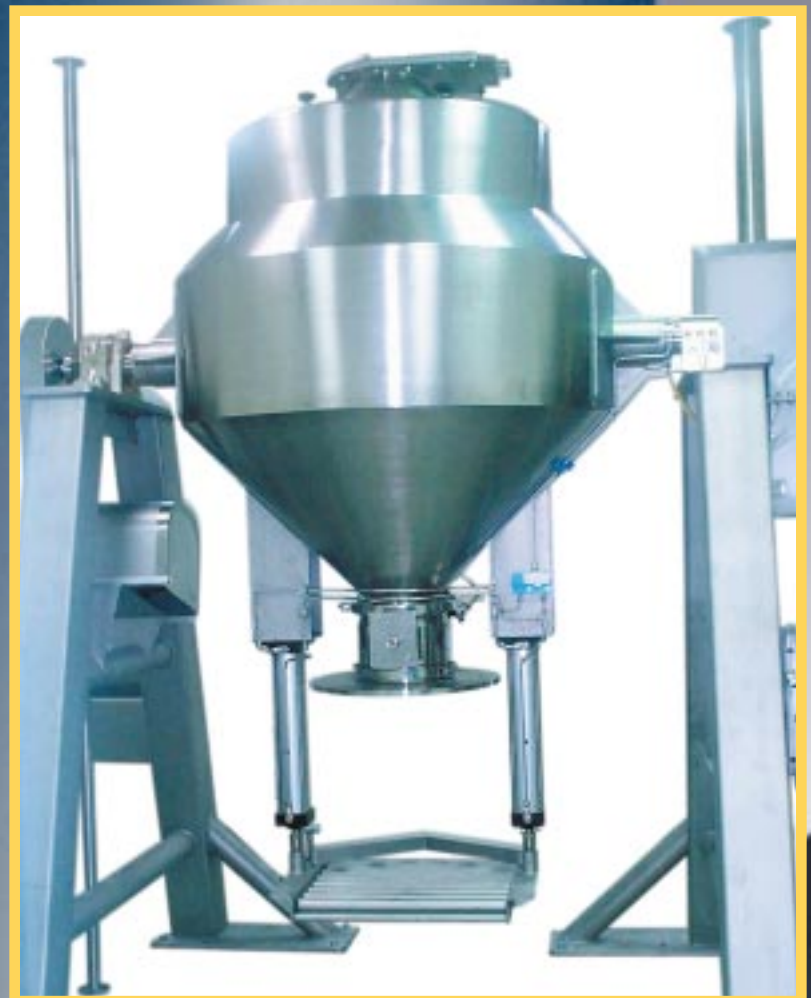
Conical Blender with Automated Drum Loading System
