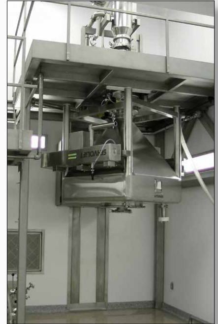
Unit buried in wall with High Containment docking from above
