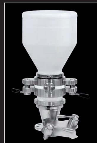
Due to the unique properties of the PTFE seal the valve can be used for charging both powders and liquids. A full range of customised charge drums are also available in stainless steel, PP, PTFE or HC22 complete with integrated spray nozzles to ensure a complete charge.
